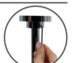
Ensuring the rubber washer is in the correct position, attach the shower head to the fixed arm and carefully secure using a suitable spanner, or a tool with smooth jaws, sufficiently to lock the head into position.
