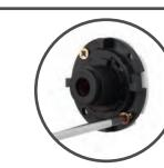
Place the 'O' ring on the recess of the spigot section on the mounting plate, offer the wall outlet onto the mounting plate in the 5 o'clock position and rotate clockwise until a stop is reached.
